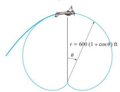
When an airplane executes the vertical loop shown above, the centrifugal force causes the normal force (apparent weight) on the pilot to be smaller than her actual weight.
