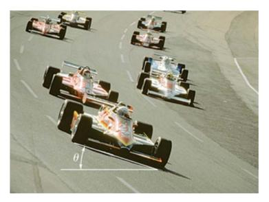
Race track turns are often banked to reduce the frictional forces required to keep the cars from sliding up to the outer rail at high speeds.
