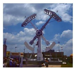
This picture shows a ride at the amusement park. The hydraulically-powered arms turn at a constant rate, which creates a centrifugal force on the riders.
