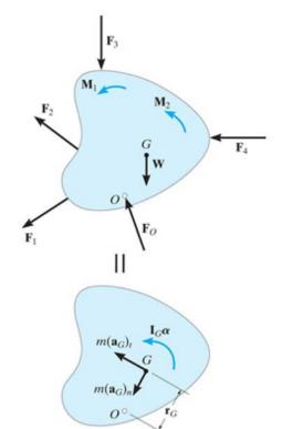
From the parallel axis theorem,  $I_O = I_G + m(r_G)^2$ , therefore the term in parentheses represents  $I_O$ .
