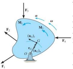
When a rigid body rotates about a fixed axis perpendicular to the plane of the body at point O, the body's center of gravity G moves in a circular path of radius  $r_G$ . Thus, the acceleration of point G can be represented by a tangential component  $(a_G)_t = r_G \alpha$  and a normal component  $(a_G)_n = r_G \omega^2$ .
