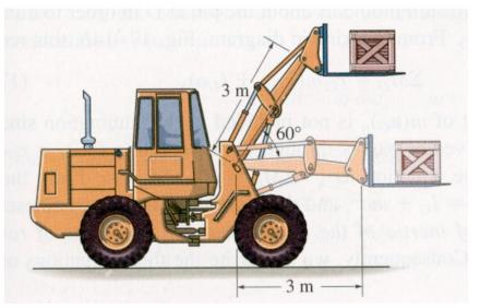
As the tractor raises the load, the crate will undergo curvilinear translation if the forks do not rotate.
