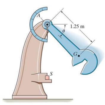
The pendulum of the Charpy impact machine is released from rest when  $\theta = 0^{\circ}$ . Its angular velocity ( $\omega$ ) begins to increase.
