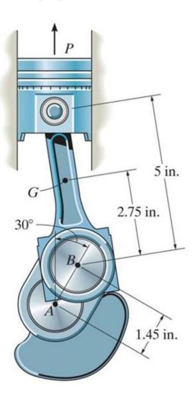
In an automotive engine, the forces delivered to the crankshaft, and the angular acceleration of the crankshaft, depend on the speed and acceleration of the piston.
