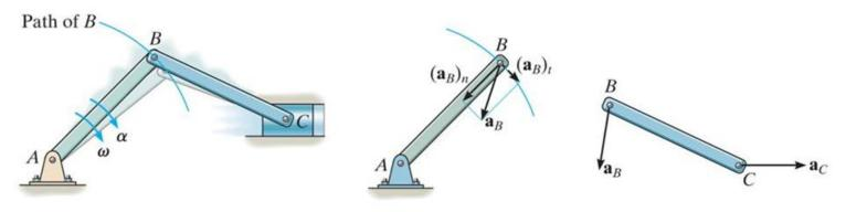
In this mechanism, point B is known to travel along a circular path, so  $\mathbf{a}_{B}$  can be expressed in terms of its normal and tangential components. Note that point B on link BC will have the same acceleration as point B on link AB.
