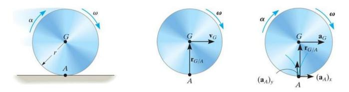
As the cylinder rolls, point G (center) moves along a straight line. If  $\omega$  and  $\alpha$  are known, the relative velocity and acceleration equations can be applied to A, at the instant A is in contact with the ground. The point A is the instantaneous center of zero velocity, however it is not a point of zero acceleration.
