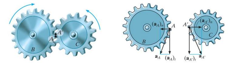
In this case, the tangential components of acceleration will be the same, i. e.,
