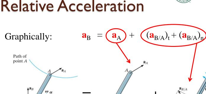
The relative tangential acceleration component  $(\mathbf{a}_{B/A})_t$  is  $(\boldsymbol{\alpha} \times \mathbf{r}_{B/A})$  and perpendicular to  $\mathbf{r}_{B/A}$ .
